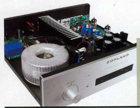
Copland's high standards of 'look' and 'feet' are obvious from the outside the CSA29 amplifier, which still features those classic 'Cello-style' control knobs Inside, its a heavyweight, with a massive toroidal transformer and reservoir capacitors as well as substantial heatsinks for the MOSFET output devices. The two input-stage tubes are seen to the right
